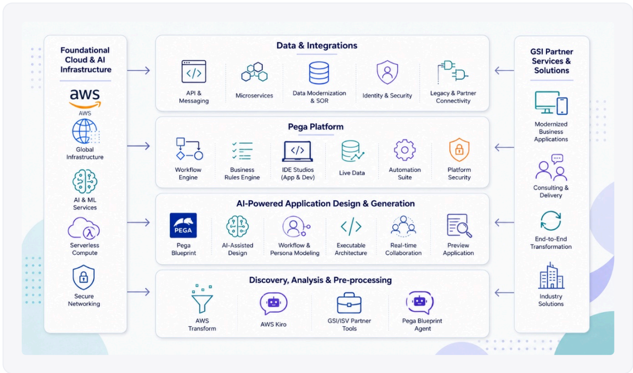
Figure 2: Anatomy of the AI-Driven App Modernization Platform: The platform's architecture integrates Pega and AWS pillars with four horizontal processing layers. The engine flows from the AWS foundation upward, sequentially analyzing legacy assets, designing the new application in Pega Blueprint, and generating it on the Pega Platform, all while supported by a universal data and integration layer and is crowned by the GSI Partner Services layer, which ensures expert delivery and business value realization.
