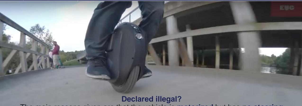
The main reasons given are that the vehicle is **motorized** but has **no steering** wheel and **no place to sit**. Therefore, the vehicle does not fall in any category allowed.
